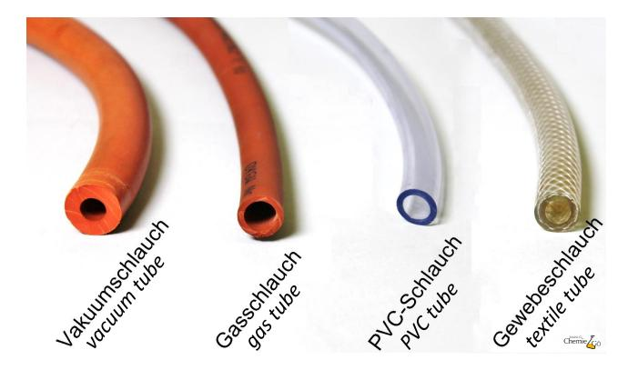
A vacuum tube is used as the connection between the inhouse vacuum or a vacuum pump and the experimental apparatus.
