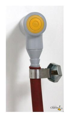
PVC tubing is used to transfer gas or liquids as well as in the cooling water circuit.
