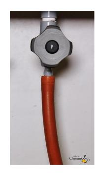
Rubber tubes can be used e.g. as the connection between the gas valve and the gas burner.
